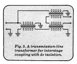
3B.) Even though one leg is still grounded at each end, the ground current will be impeded by inductive reactance. The transmission-line currents, however, would not be affected here because they are equal and opposite at every point along the line, thus neutralizing the inductive effect of the coil. The actual line length can be short as 1/50-wavelength so no significant phase shift takes place.
